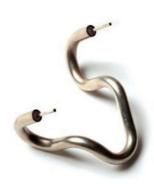
The most popular product lines for space flight cable are the UTiFLEX MCJ type constructions incorporating KEVLAR® based metalized fibers called ARACON®. This ultralight, stronger than steel material provides tremendous opportunities for weight savings without a sacrifice in performance over conventional coaxial cable. These lighter coaxial cables, with the lowest loss per gram of mass, are a critical component to reduce launch costs or increase payload capacity for many satellite customers.
